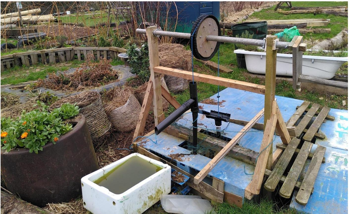
**Above:** Rope pump, constructed by Duke of Edinburgh Award volunteers with some adult guidance too. Please [click here](#) to see the rope pump in action. It's an inspirational sustainable example of how to pump rainwater to the surface using an inverted motorbike tyre, some rope and rubber washers from an old tyre.
