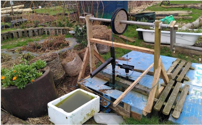
**Above:** Rope pump, constructed by Duke of Edinburgh Award volunteers with some adult guidance too. Please <u>click here</u> to see the rope pump in action. It's an inspirational sustainable example of how to pump rainwater to the surface using an inverted motorbike tyre, some rope and rubber washes from an old tyre.
